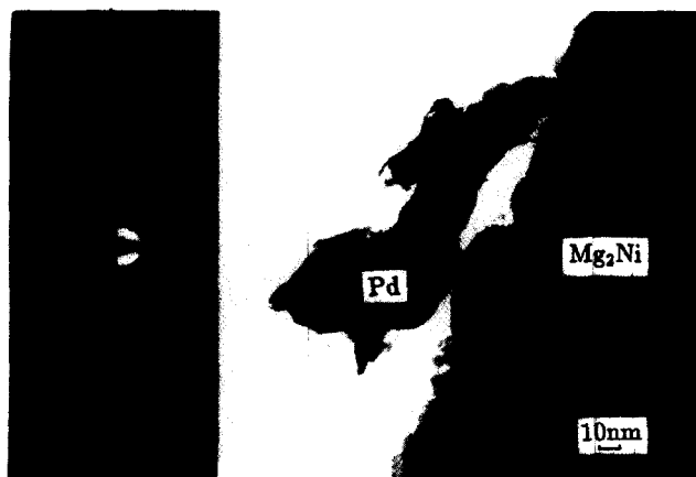
Fig. 6. TEM image of nanocrystalline Mg 2 Ni with Pd, and electron diffraction pattern of Mg 2 Ni.
